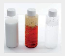
Stable tank mixes form milky emulsions, like those in the container on the left in the photo above. When using liquid nitrogen as a carrier, the addition of compatibility agents, like Convert™, can prevent tank mixes from quickly separating and leaving residues trapped inside the tank. Convert can reduce the risk of cross contamination and lower levels of weed control.
