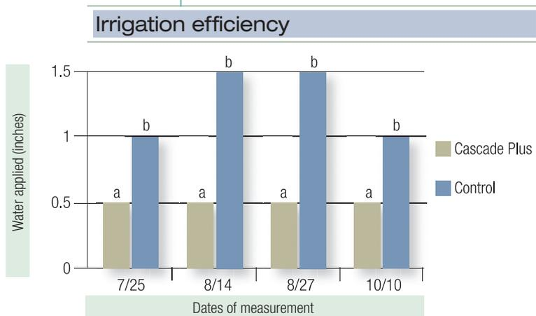
**Figure 1.** Amount of water required to bring soil moisture content up from 5% to 15%. Different letters at each observation date indicate a significant difference between the Cascade Plus treatment and the control.
