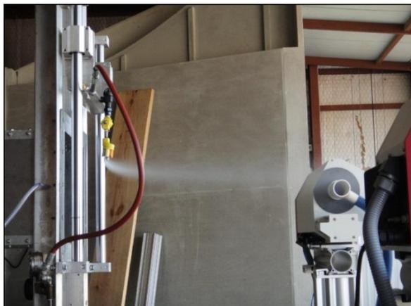
**Figure 1.** Wind tunnel outlet, nozzle mount and traverse and laser positioning.
